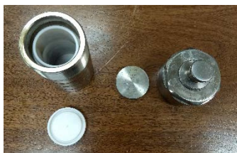
Figure S1: Stainless steel autoclave vessel with Teflon coated container inside.
